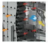
Drying occurs in the tiers of the Sukup Full-Heat Mixed-Flow drver. Each tier has a row of inlet ducts open to the center of the dryer and a row of exhaust ducts open to the outside of the dryer. Hot air from the fan & heater enters the inlet ducts and moves through the grain in mixed directions to the nearest exhaust ducts. This gives more even drying air temperature to all the grain in the dryer, resulting in better fuel efficiency and grain
