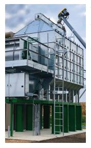
Low-speed centrifugal fans make the dryer very quiet.
